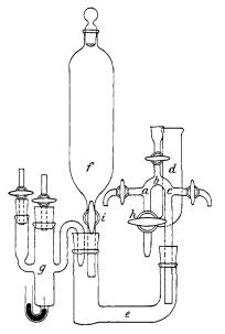
gether. Stopcocks a, b and c are opened and the solution is drained.
